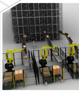
Cases of product are released from the Multishuttle order fulfillment sequencing buffer and are palletized using robots.
