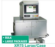
With a 620mm belt width, the heavyduty XR75 Large has ample capacity to inspect end-of-line cases. It can also be configured for large-width bulk format applications.
