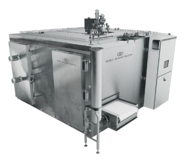
Continuous, in-line, linear tunnel designed to individually quick freeze products, optimize production capacity and preserve long lasting quality.
