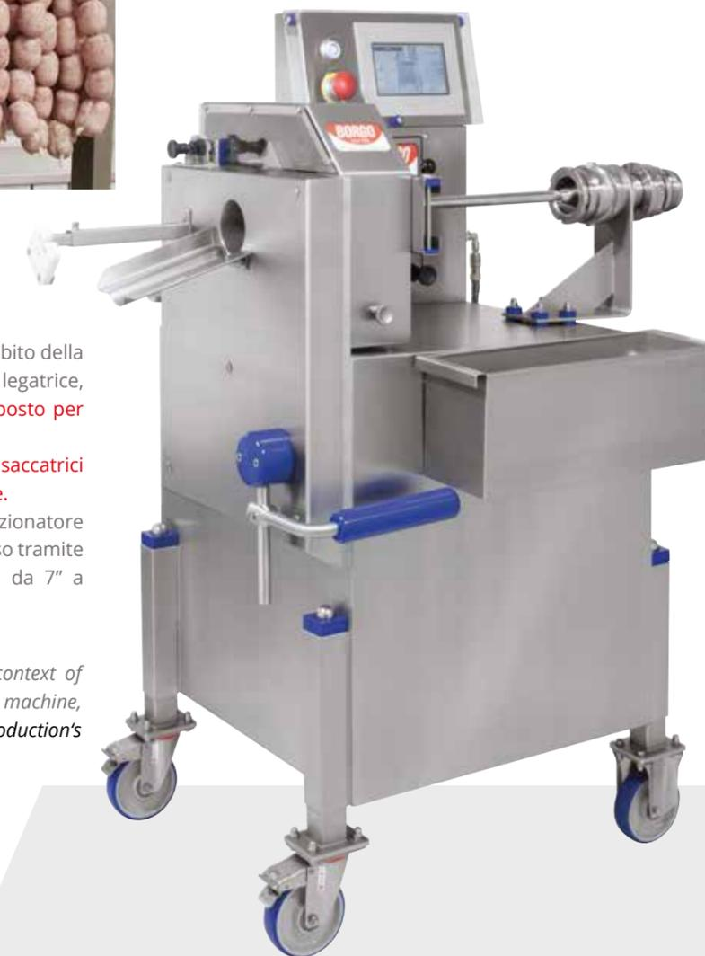
**Easy to clean**, by the openings of the various covers, it allows you to access easily even the most difficult parts. **Construction in stainless steel, smooth finish, inclined planes, raised from the ground.**
