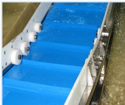
SuperDrive™ with Flights Working under Water
