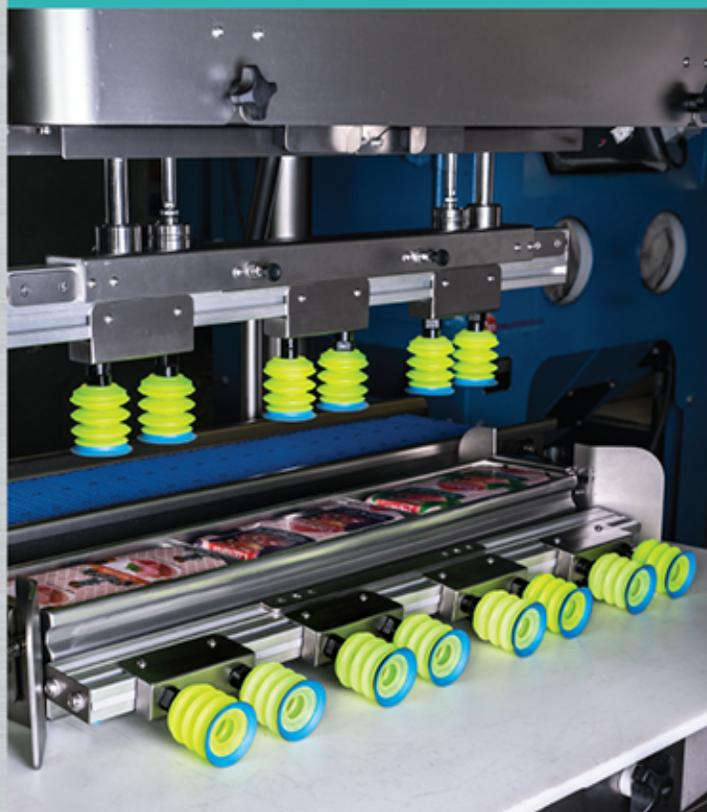
Depending on format or product size to be demoulded, stuckers holder head can be replaced to get a better position and center of the stuckers for each ham (6 or 8 stucks head).
