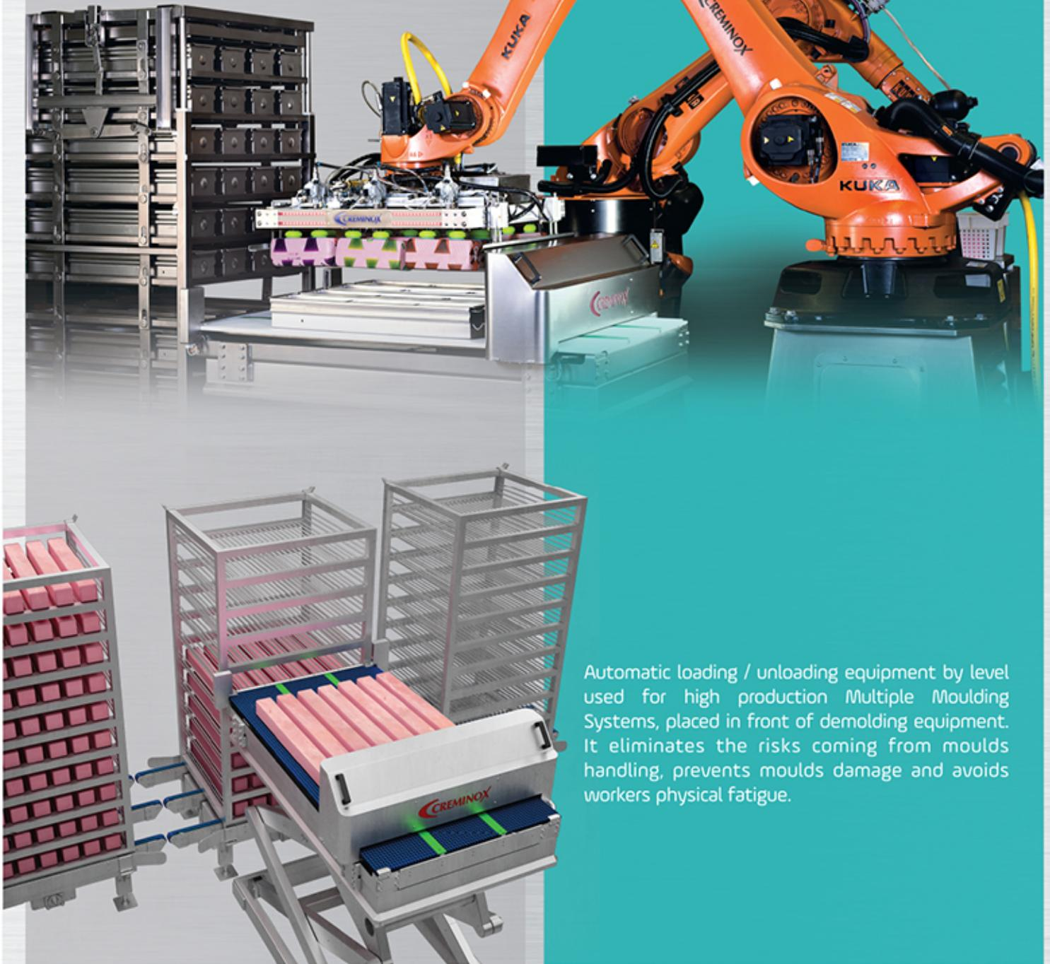
Automatic loading / unloading equipment by level used for high production Multiple Moulding Systems, placed in front of demoulding equipment. It eliminates the risks coming from moulds handling, prevents moulds damage and avoids workers physical fatigue.
