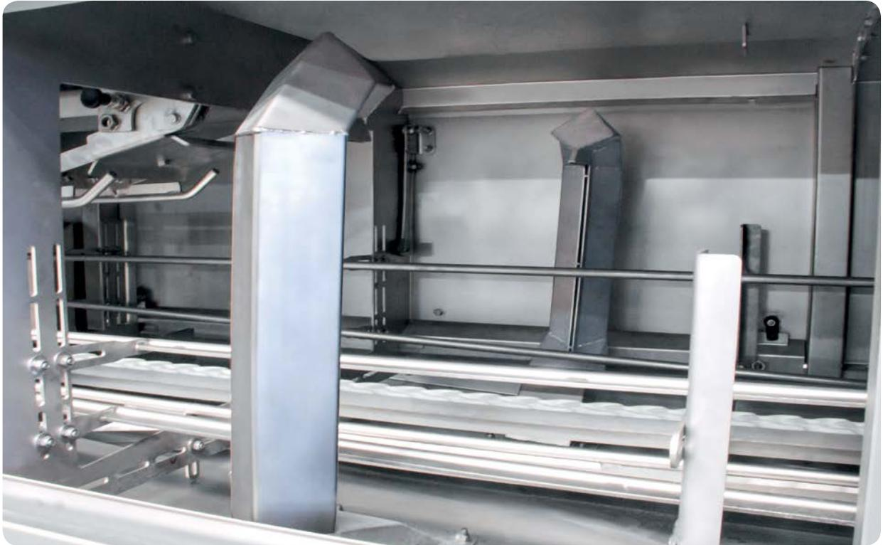
*The inner workings of the EAB-1-ST, the air blades 'cut' the residual water from the crate.*
