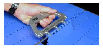
Enables simpler, faster, and safer belt installation and removal in a solid metal, handheld tool
