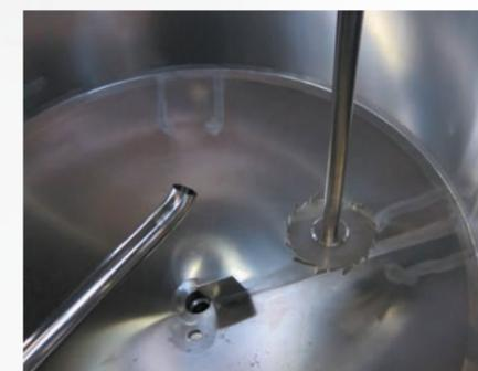
High speed crushing propeller
