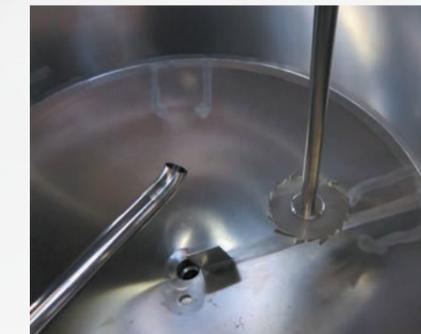
High speed crushing propeller
