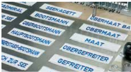
STENCIL FRAME With 24 production panels. Panel size 113 x 28 mm / 4.44" x 1.1"
