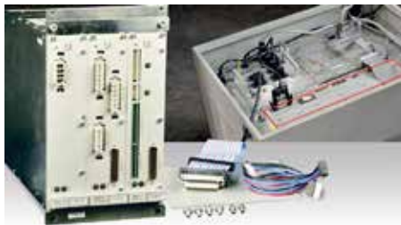
UPGRADE FOR POWER DRIVE With this power module it is possible to change a single circuit board. In case of a damage it is not longer necessary to change the whole unit.
