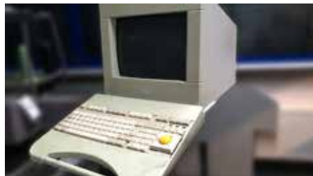
UPGRADE MSCA MONITORS MSCA monitors can be upgraded with a TFT upgrade kit. The monitor gets replaced by a cable and a cover.
