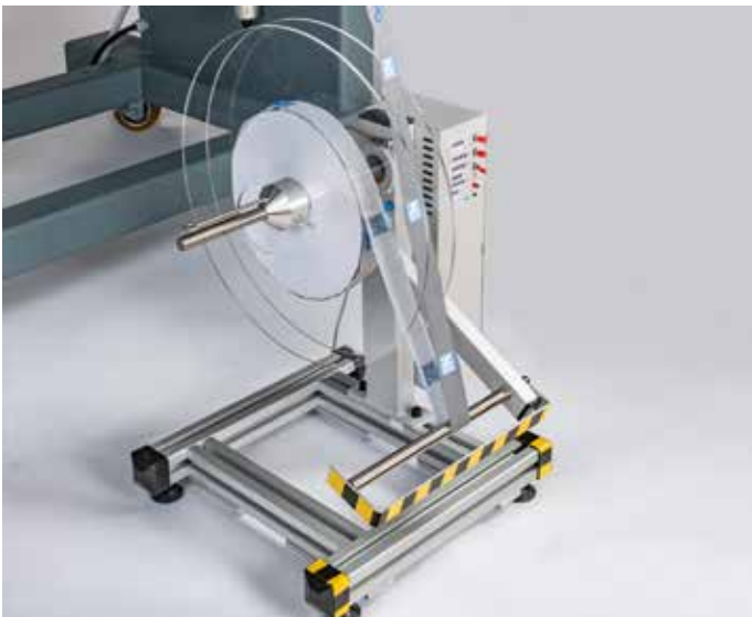
ROLL2BASKET UP WINDING UNIT FOR ROLL2BASKET The embroidered ribbon is wound onto a roll for further processing. For rolls with up to 400mm diameter and materials of up to 5mm thickness.
