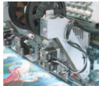
■ Double Twin Sequin Device ● 双侧双珠片装置
