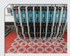
High precision sequin feeding, sequin gap reach to 0.1mm, color overlap accuracy, minimum gap reach to 0.05mm, not easy missing sequin and turn over sequin.
