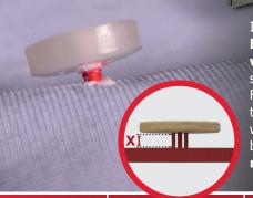
In order to achieve a consistently high standard of button shank wrapping it is essential that the shank length (X) is of sufficient length. Failure to achieve this will reduce the yield per cone and render the wrapping less effective in securing the button. This is a simple setting on most button attaching machines.
