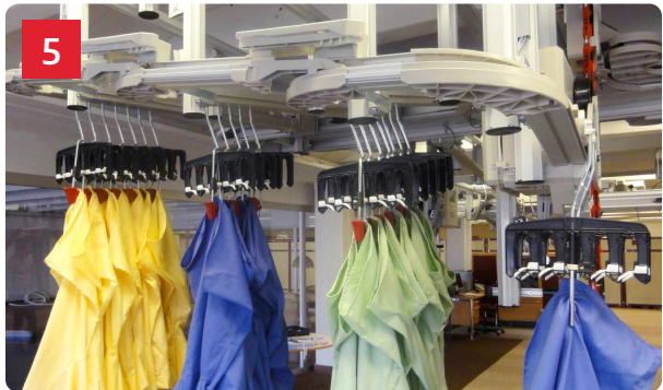
5 Multi-rail stations can automatically both sort and buffer products within a workstation. This maximizes operator productivity.
