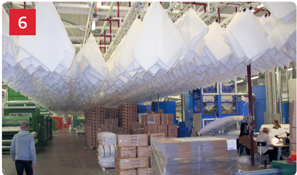
Overhead feeding buffer for optimal utilization of space.
