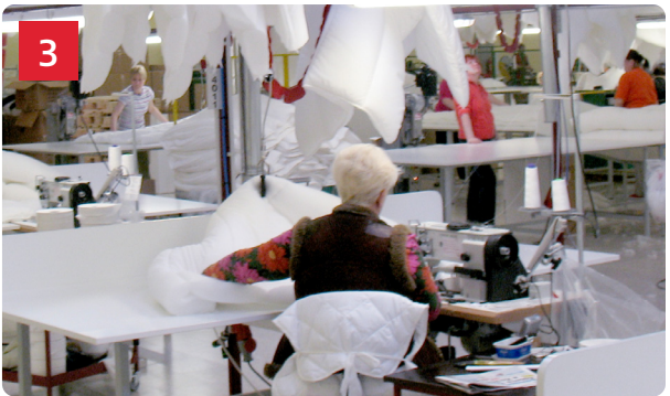
High efficiency thanks to the chain. Most of the operations can be performed without removing the product from the product carrier.
