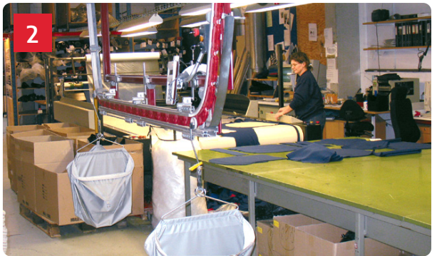
Tailored workstations and customized carriers are incorporated with RFID technology that automatically generates information for the Eton select software.
