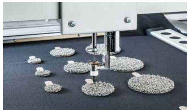
ZSK's K head technology creating sensors with conductive yarn.
