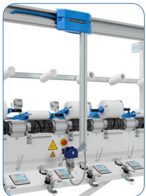
Splicer montato su rotaia Splicer mounted on rail Splicer montado sobre riel Splicer monté sur rail Splicer auf Schiene
