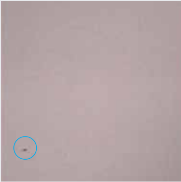
Hole Defect in Plain Fabric
