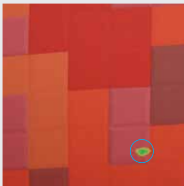
Weaving Defect in Patterned Fabric in Heat Map
