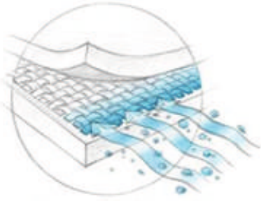
Classic layers do not prevent water ingress
