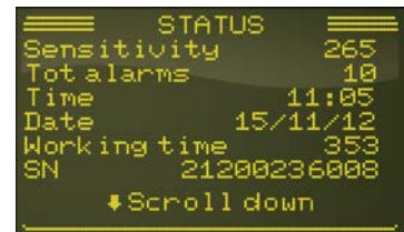
Display of the status of the metal detector
