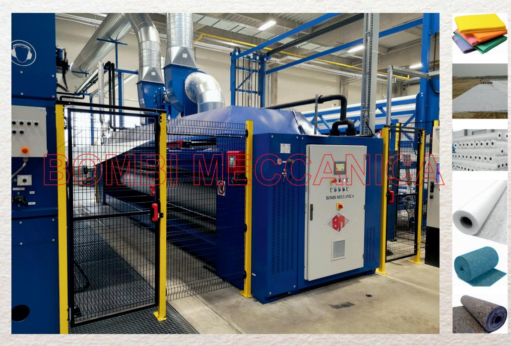
A hot calender is the simplest and most effective solution to transform a standard needled punched felt into a **high technical product**, giving immediate benefit and extra added value. This is achieved **without any modification within the existing line.**
