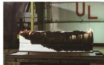
Mattress made of Yilun fiber, flaming after 30 minutes
