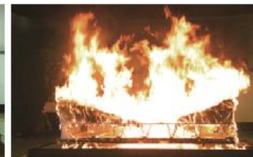
Mattress made of normal fabric, flaming after 4 minutes
