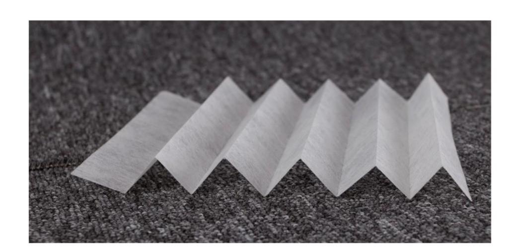
Ultrasonic composite filter media can be imprinted by all kinds of patterns. The middle layer is PP electrostatic melt-blown fabric which can absorb the dust strongly and conforming to the environmental requirement.
