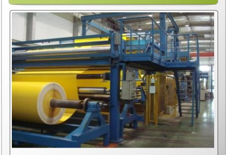
Hot-melt coating line KKA from Germany; Knife coating line ISOTEX from Itlay.
