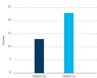
Comparison of the rundown-times of both types yarn guide roller generations
