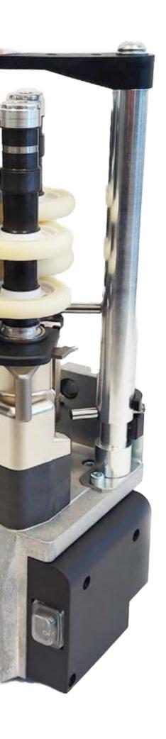
Simple and Fast Changeover of S/Z Yarn Twist Directions
