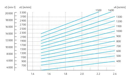
Yarn running speeds VA [m/min] and disc speeds ns [min-1] in dependence on D/Y:
