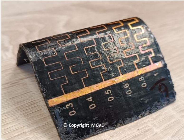
Organosheet PA with printed circuit Cu tracks by MCVE
