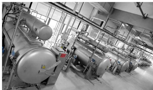
**The jet dyeing machine AcquaZero® (both MF and reel less SP model)** allows higher flexibility and up to 50% water saving versus conventional machines.
