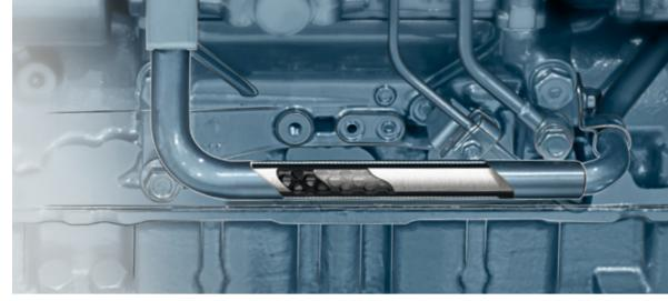
Multiple layers of support and filter sleeves for oil filters
