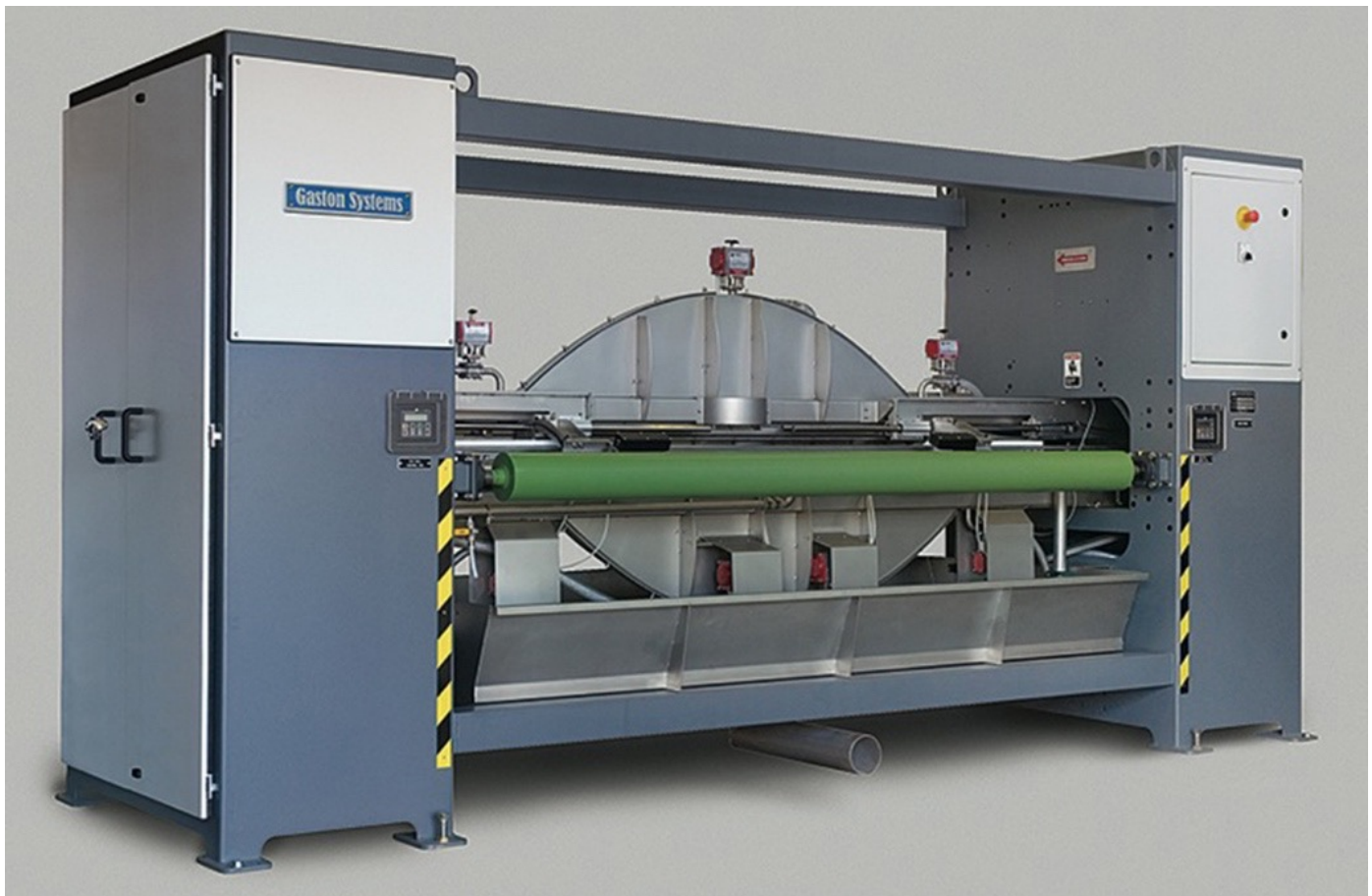
Low moisture Foam Applicator achieves exact, uniform application of chemicals to open-width substrate
