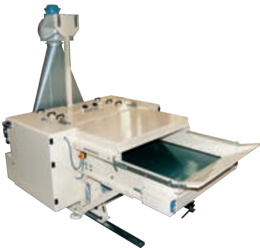
BTO 1300 TRIM AND ROLLS OPENER WITH BIT REMOVAL
