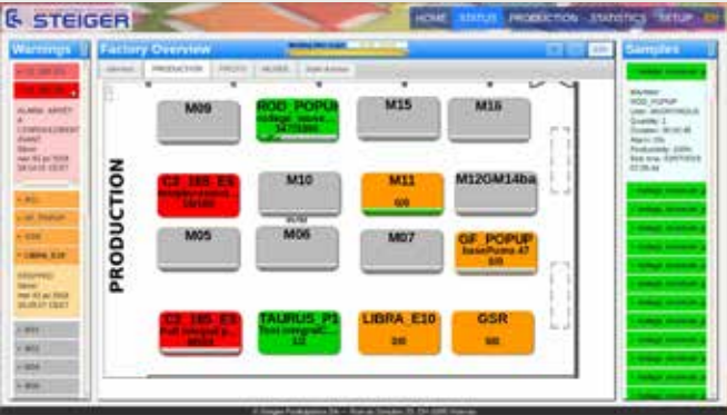
Display of the shop-floor with machine status
