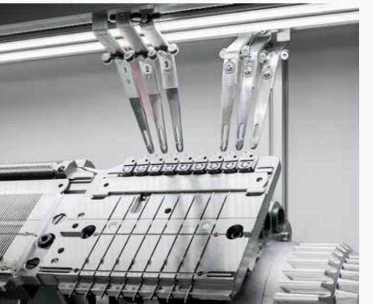
The new clamp and scissor system ensures that the yarns of the yarn-carriers are independently gripped. Gears prevent the yarn from escaping and guarantee the correct yarn gripping or cutting. High intensity LED ribbons illuminate the needlebed and highlight the formation of the stitch.
