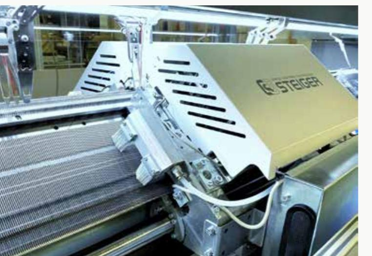
Short, light, the **cam-box** has been designed exclusively for medical application. Combined with the new **dynamic electronic drive system**, the acceleration and deceleration performances of the cam-box have also been enhanced. In order to support this increased carriage reactivity, Steiger has also strengthened the **stiffness of the main frame**.
