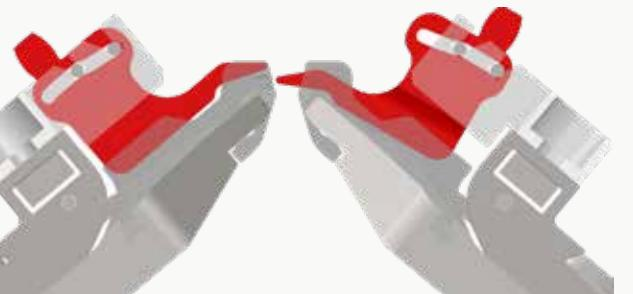
The main innovation arises from a completely new sinker system. The perfect guiding of the sinker using a sinker bed and a new activation system has resulted in an optimal maintaining of the elastic yarn during the creation of the stitch. No elastane is knitted together with the base yarn even with an increased production speed. This function is programmable. During a knitting row it can be activated or deactivated several times according to the defined program.
