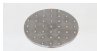
Example of 1-position sample holder for leather and coated fabrics
