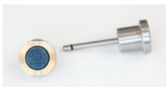
Example of 1-position sample holder with Ø 38 mm
