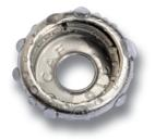
Hardly anybody realizes that press fasteners used in the tough conditions like marine applications are not even resistant to sea water - until now. Probably the smallest item on deck is now available in real 316 stainless steel: CAF-316°. To achieve true durability, even the internal spring is made of top quality duplex stainless steel, insuring years of dependable performance regardless of the conditions.
