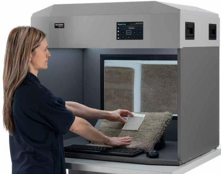
In the same operation, physical samples can be assessed visually in precisely controlled LED viewing conditions and compared with a digital standard image taken in a DigiEye imaging system.
