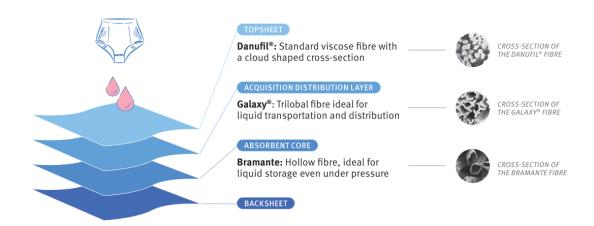
Schematic representation of the liner developed by Kelheim and Gebr. Otto for period underwear.
