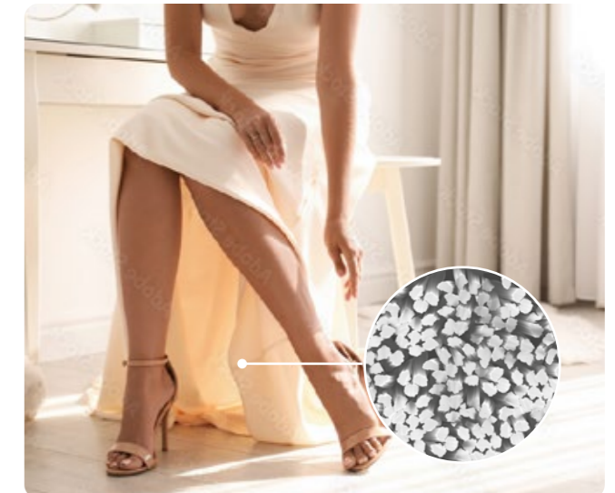
Microscopic image of a yarn made of 100% VISETA® with fine and dense fibre spacing.
