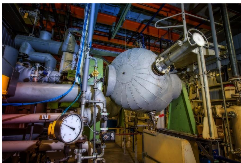
Figure 4. Pilot plant scale SSP reactor
