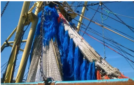
2019/20: large scale test marine degradable dolly rope
