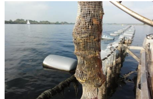
Test stage: Marine degradable mussel socks
