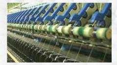
**Ring spinning**: The setup at SGL comprises of the latest and advanced machinery imported from Spain, Japan and China to produce fine quality yarns. Ring frames equipped with Steel, Glass and Spandex core attachments produce robust high-performance yarns.
