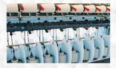
**Plied yarns** are also produced by Two-for-one twisting mechanism for customized product development within the facility by using state-ofthe-art technology from Japan.
