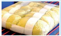
Automatic packaging of balls in one level into pre-manufactured plastic bags. Available with labelling device for barcode labels.
