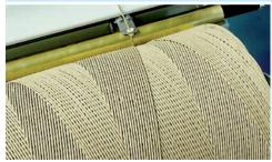
Precision cross winding machine for all kinds of coarse yarns, coreless or on tubes. Electronic traverse motion for flexible setup of all working parameters.
