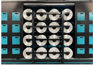
**Ra Vision** is an automatic instrument for the first visual control of the yarn bobbins produced into the spinning process (extrusion and takeup winders) to identify possible problems and evaluate the quality of yarn bobbins. Within the same system it can find all types of visual yarn bobbins defects.
