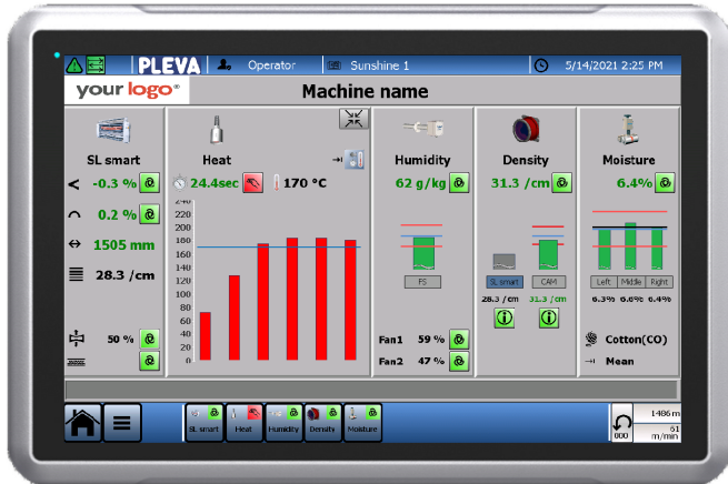
HMI with individualizable overview-page (SL smart with options for process control)
