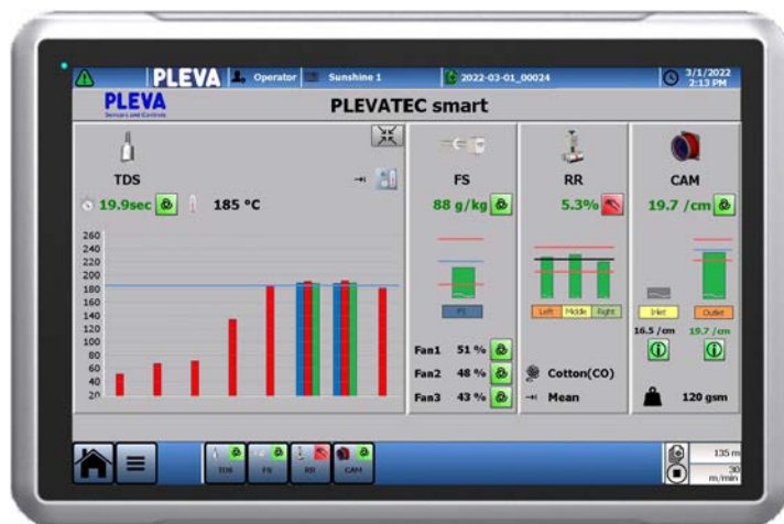
HMI touch panel with individualizable overview-page
