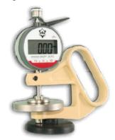
We offer special designs for textiles, fleece and leather. In accordance with applicable standards, these special designs apply defined test pressures to a fixed, circular test surface. In order to guarantee the test pressure at all times, these devices are only available with a stand.
