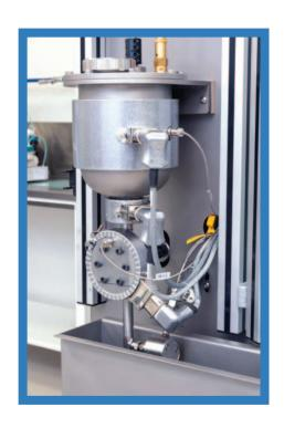
**4.1**Multiple dope vessel sizes available with temperature control and homogenised stirring capacity
