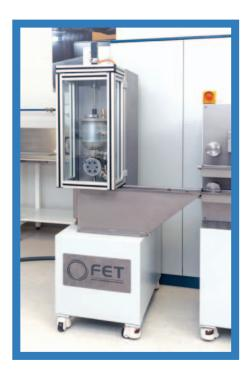
**4.2** Spinneret holder optimises extrusion into coagulation tank
