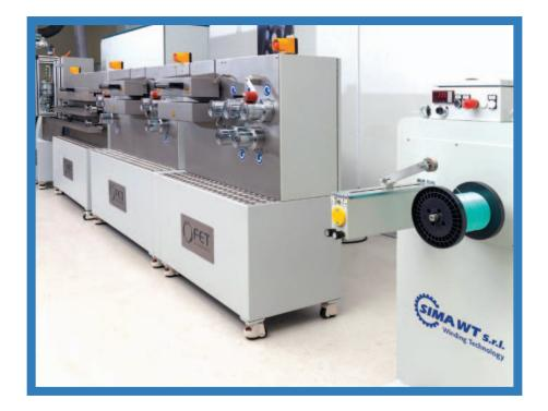
**4.5**Various take-up systems available, including flange-spool type, precision cross-winding and high-speed versions
