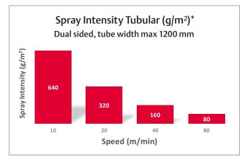
\*The exact coverage on fabric is depending on the fabric characteristics. Chemistry to be formulated for spray application with maximum viscosity at 8mPa · s.
