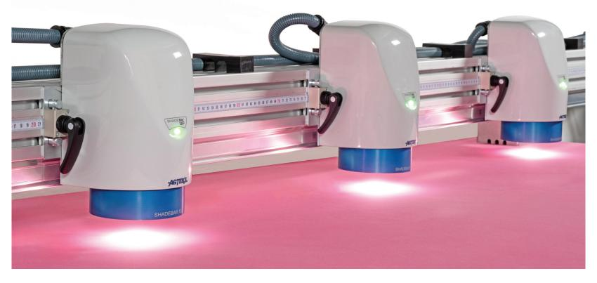
**ShadeBar** can detect longitudinal, edges, and middle color differences as an online operation.
