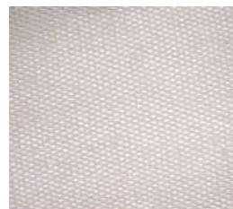
8330 Meta-Aramid Mesh Weight: 100-106g/m 2 Width: 198-203cm
