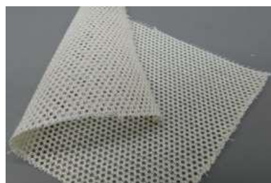
8730 Meta Aramid Mesh Weight: 105-115g/m 2 Width: 220-225cm
