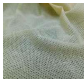
8730 Meta Aramid Mesh Weight: 105-115g/m 2 Width: 220-225cm
