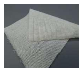
5300 Aramid Mesh Weight: 140g/m 2 Width: 100cm
