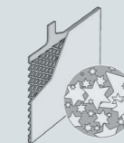
Without Carbon Boost® The plates are covered with sulfate
