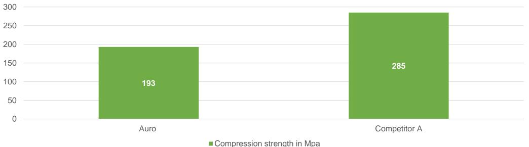
\*Compression strength results are based on the basis of tests performed at IIT, Delhi Auro Clutch Facings are designed to provide the Optimal Compression Strength, maintaining the same at the given level offers us advantages in Burst Strength and Brittleness.
